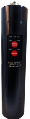
Figure 4: ReferenceMate portable shaker
