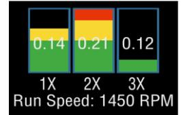
The display shows the vibration level in frequency ranges based on multiples (1X, 2X and 3X) of the specified machine run speed shown beneath the bars.
