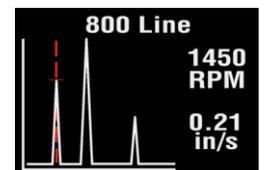
Press the down arrow to increase the resolution of the frequency axis from 100 (10 Hz or 600 RPM resolution) to 800 lines (1.25 Hz or 75 RPM resolution). Increasing the resolution zooms into the frequency spectrum. Scroll using the arrows to display the full spectrum at the higher resolution.
